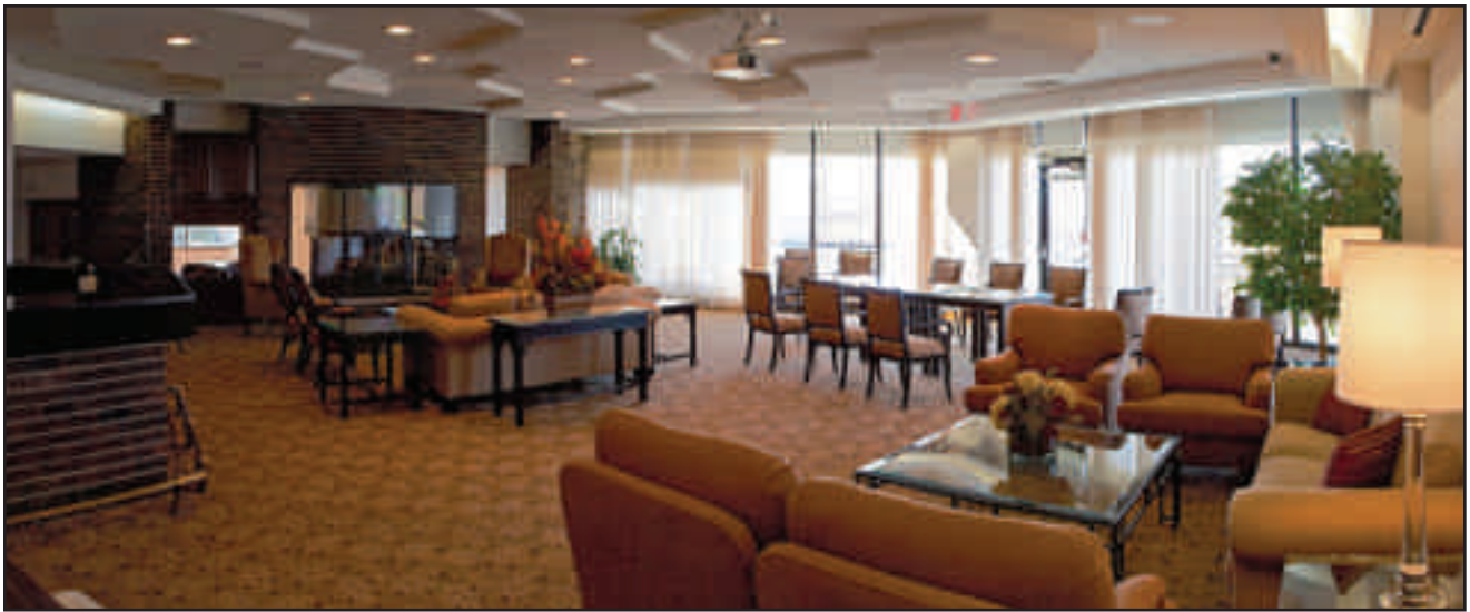
The new lighting in The Masters' Clubhouse Lounge. It is on "passive infrared and microphonic sensors" and shuts off if no one is in the room for 10 minutes.
